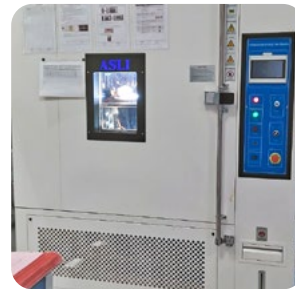
Environmental and humidity chambers
