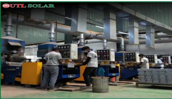
Grid casting set-up for lead acid batteries
