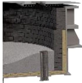
EBT Tap Hole Sleeve & Block
