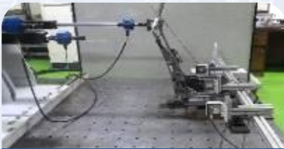
Horizontal Backward Moment Loading Test (Strength Test)
