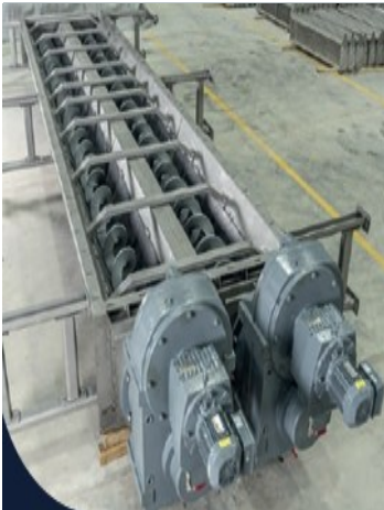
Twin Screw Conveyors for Sludge Handling
