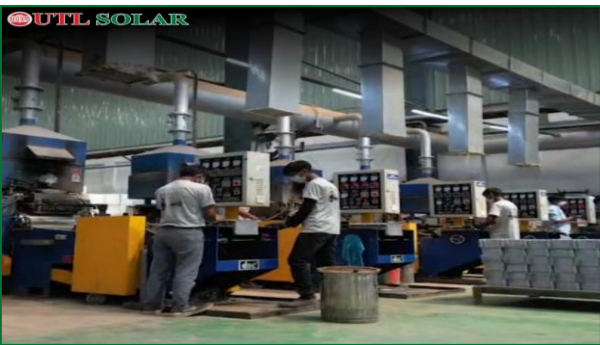
Grid casting set-up for lead acid batteries
