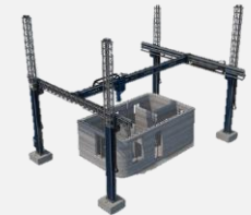
3D Concrete Printer
