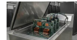
Immersion Cooled Data Centre
