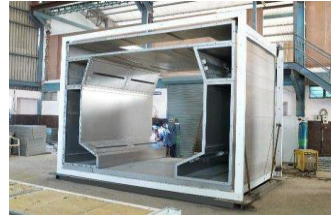
Car Paint booth
