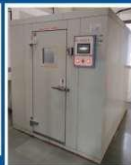
Temperature & Humidity controlled chamber for testing
