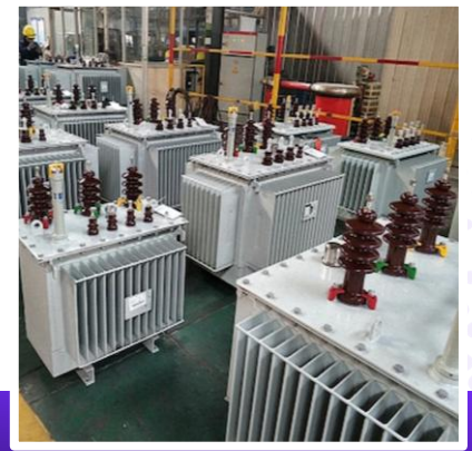
Manufacturing Of Distribution Transformers.
