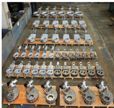
Varied Size Knife Gate Valves from DN 200 to DN 650 & Swing Gate Valve Size DN 200
