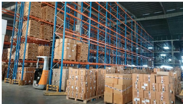
G+5 long-span pallet racking at the Bhiwandi warehouse
