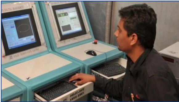
250 kV / 2,500 KVA High Voltage & PD test lab Partial discharge measurement
