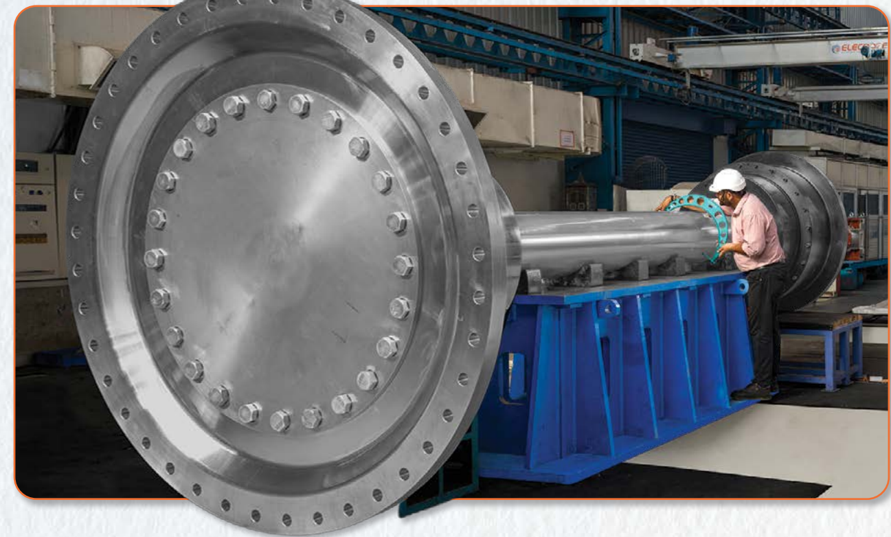
Heavy-duty geared coupling delivering 62.7 million Nm torque through a 2.35-metre diameter flange for cement mill drives.
