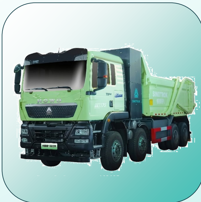
Heavy e-Tipper with swappable battery
