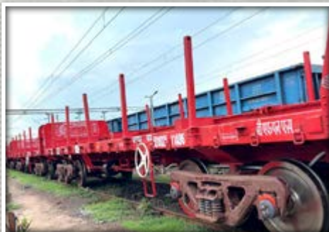
Balmer Lawrie commenced the transportation of finished steel products from SAIL's Rourkela Steel Plant using BFNS 22.9t wagons over long-haul routes. The first rake arrived at Bondamunda in Odisha on 22nd May 2025.
