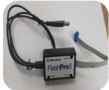
In circuit Emulator for programming of PCBs
