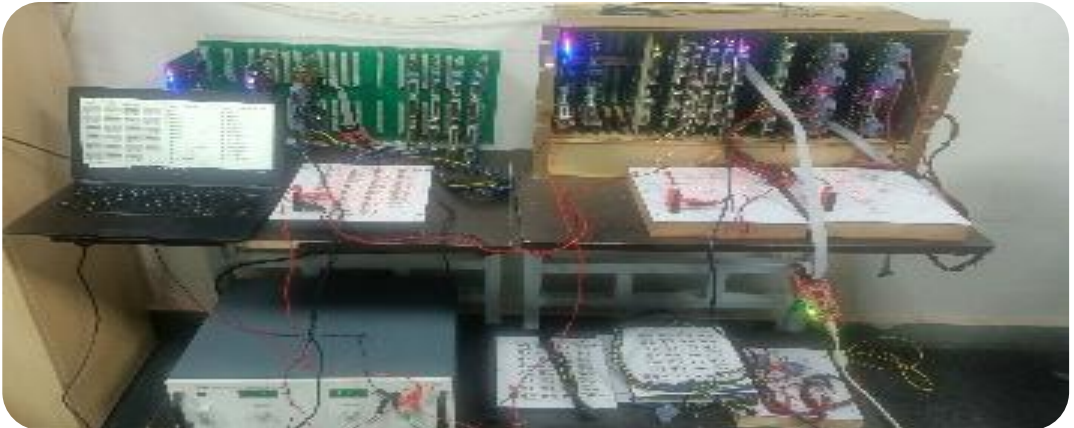
VCU Test Setup with I/O jig, simulator
