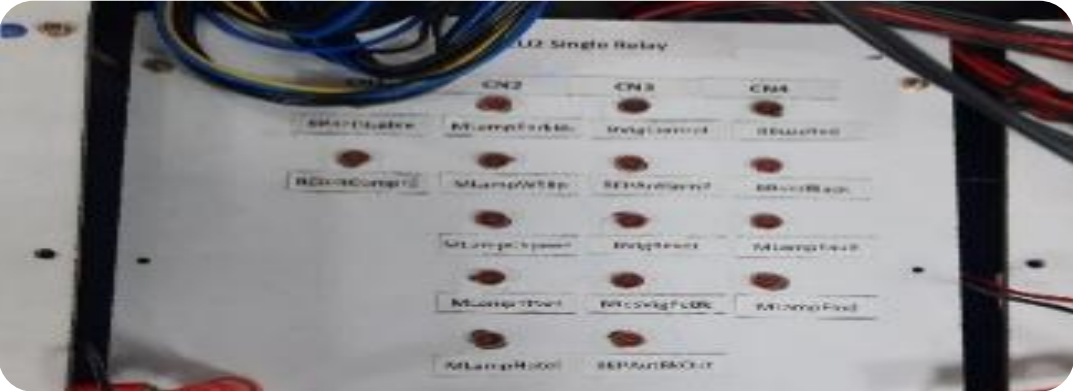
VCU Testing Jig for Digital Inputs
