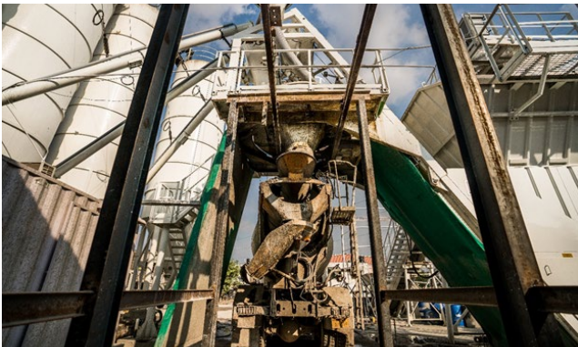
[Transit mixer being loaded at our contract manufacturing plant in Chennai]
