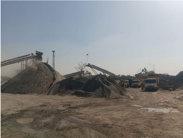
[M-Sand being produced at our contract manufacturing plant at Palamu, Jharkhand having annual capacity of 500K+ MT]
