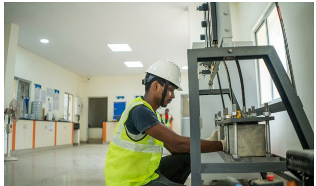
[Cube strength being tested for quality at our contract manufacturing plant in Chennai]
