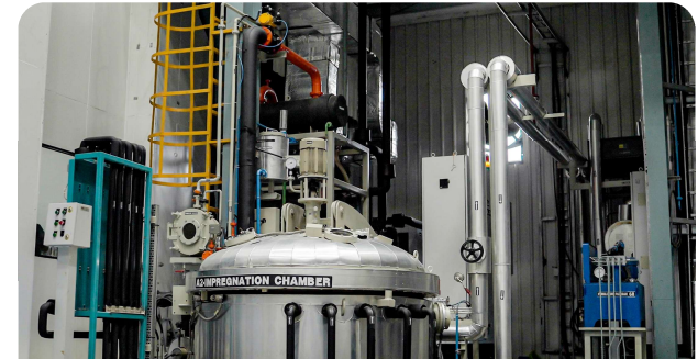
SCADA Controlled Autoclave system for fully automated vacuum drying & oil impregnation cycle Management.
