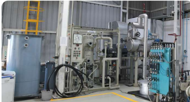
Fully integrated Oil Storage & Handling system with online re-filtration for efficient oil management to produce large batches of OIP cores across all autoclaves.
