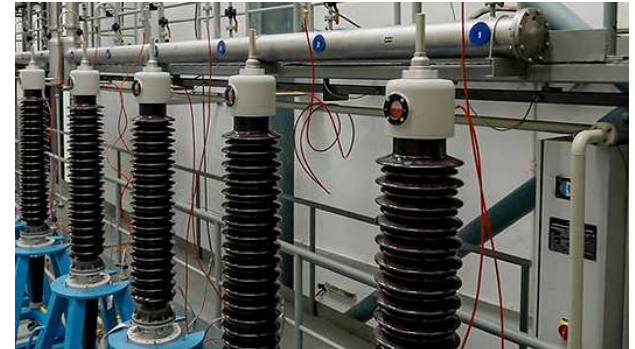
Online Oil Flooding System for automatic oil flooding & levelling, augmenting existing production capacity & process capability of oil filling under fine vacuum.
