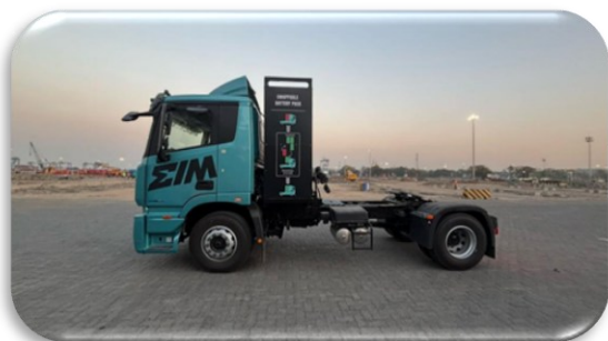
E- Tractor e-Tractor with Swappable battery pack
