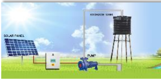
Solar Pumping System
