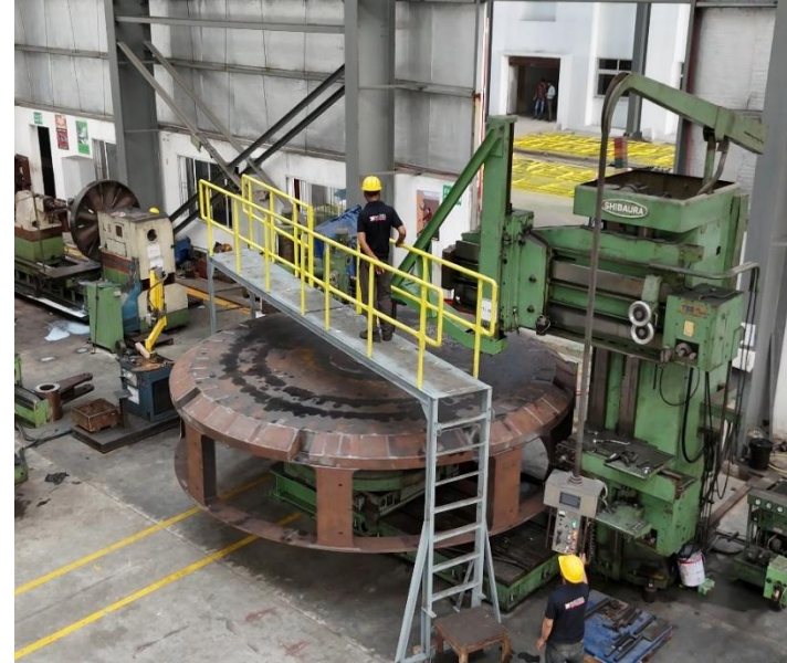
6-Meter Stacker Wheel for Limestone Mines
