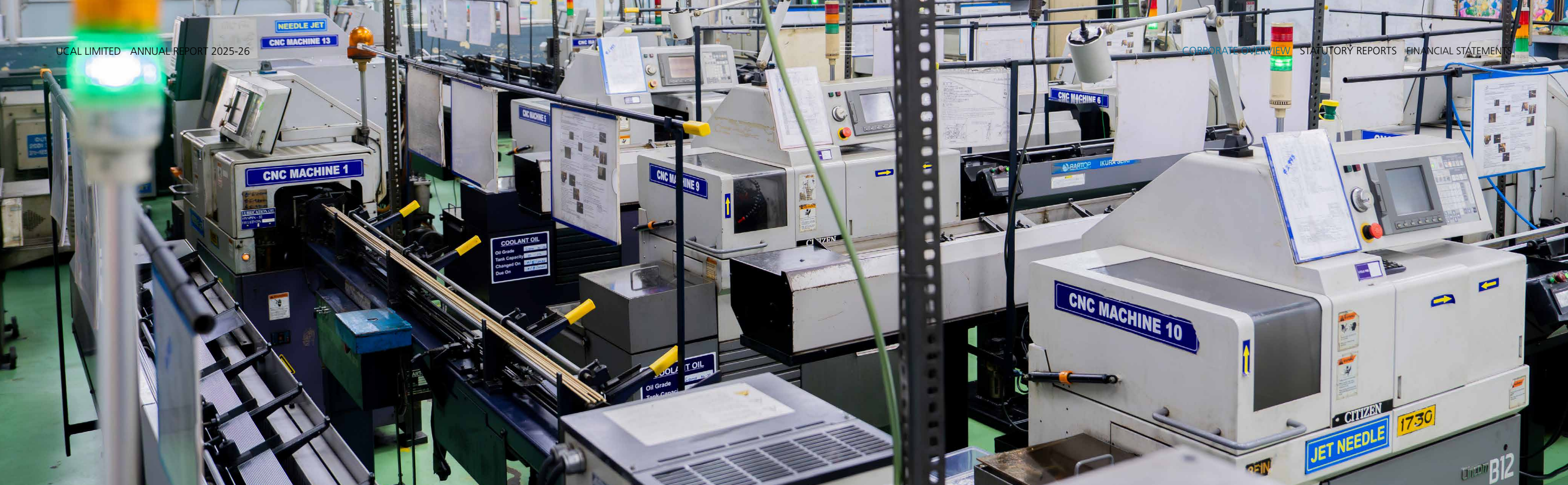
Carburettor - Precision Jet Machining Line at MM-1 Plant
