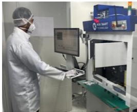
Camera Lens Active Alignment
