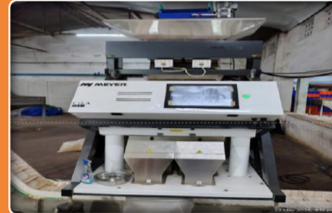
1 ton capacity color sorter for peeled cashew kernels
