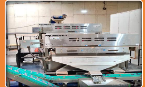
2-tonnes capacity color sorter for peeled cashew kernels
