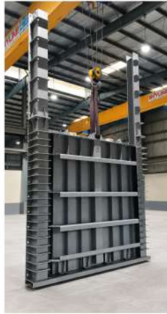
3000mm x 3000mm, Stainless Steel Sluice Gate
