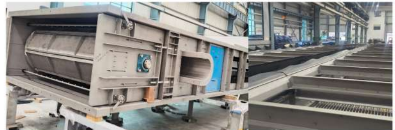
2800mm (W) x 24514mm (H), SS304 Multi-Rake Screen & 3000mm (W) x 8210mm (H), SS304 Centre Flow Travelling Band Screen
