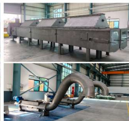
Twin Belt Conveyor with Deflector Plate Assembly, Jet Breaker, MM 2 MM Mechanical Coarse Screen
