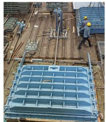
3400mm x 2400mm Cast Iron Sluice Gate for MCRP Package IV Project
