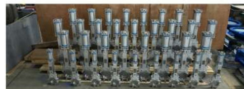
Varied Sized Knife Gate Valves of ZFI-S from DN125 to DN300
