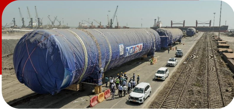
Dispatched 1 st lot of tanks of 1500 M 3 for Mini LNG Terminal of The Bahamas Project
