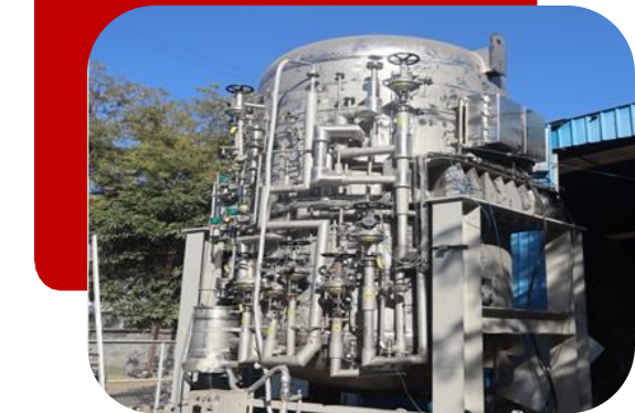
Completed the Production of complex LOX tank to be used in submarine
