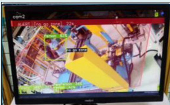
Safety Guarding with camera and AI Thermal Camera
